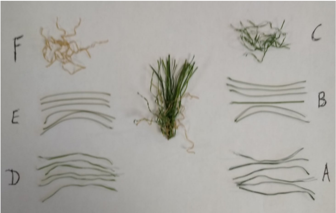
Picture 2. Build-up of the artificial grass fibers LimeGreen Landscape
