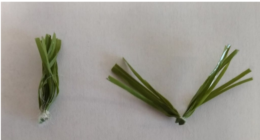
Picture 1. Build-up of the artificial grass fibers LimeGreen Play
